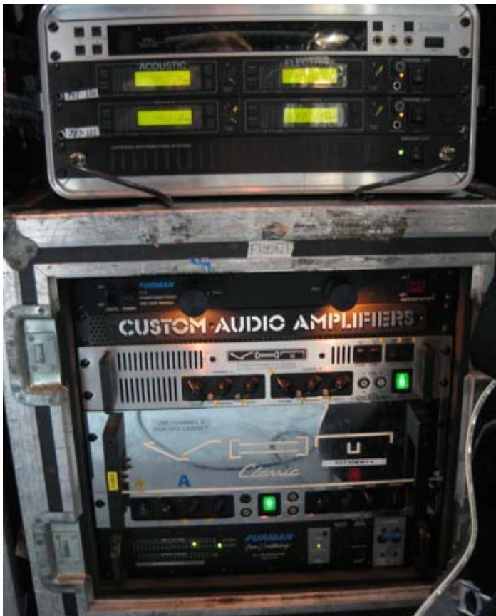
Rack 2 with wireless receivers
